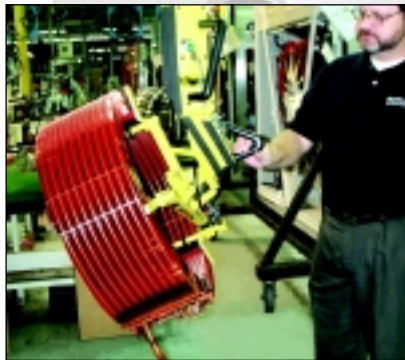
75 lb copper coil used in refrigeration container units with 90 degree rotate from Thermo King®
