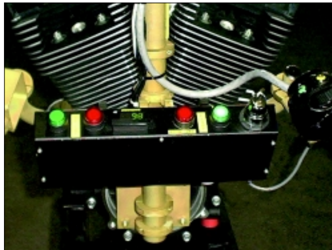
Error proof assembly: The device digitally displays the weight of the part picked up. Device will not allow the operator to move the part if not clamped properly. The key allows the operator the ability to lock the device. Allows 100% visual inspection of the assembly.
