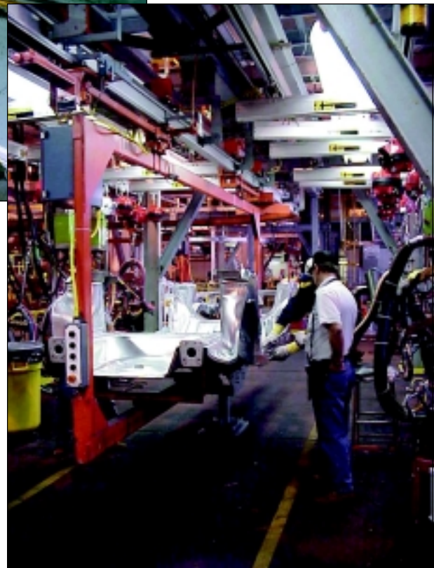
IR Zimmerman Enclosed Track Rail System: Shown here in an automotive industry application.
