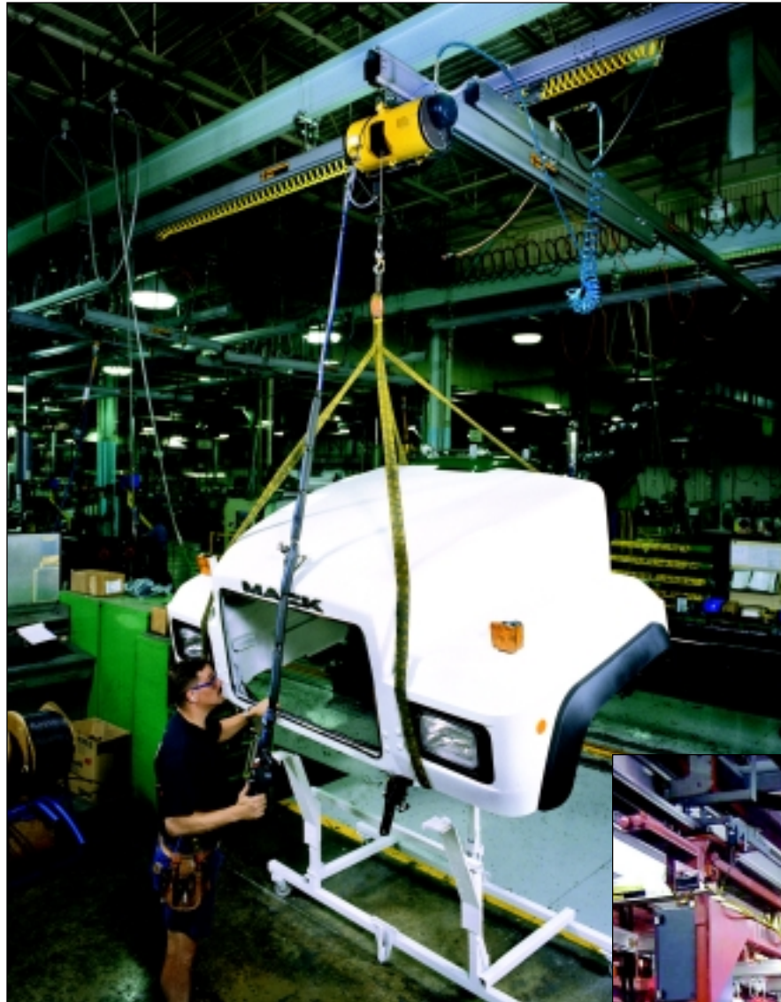
IR Zimmerman Intelligent Lifting Systems: Shown here in a vehicle assembly industry application.
