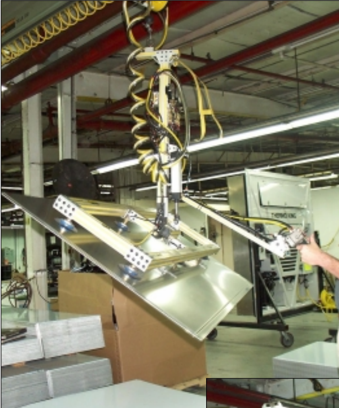
IR Zimmerman provided material handling solutions to Thermo King® in handling the back panel for a refrigeration unit. The handling device includes a Power Tilt feature.
