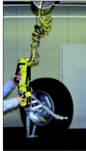
Tire handling device with 90 degree manual rotate.
